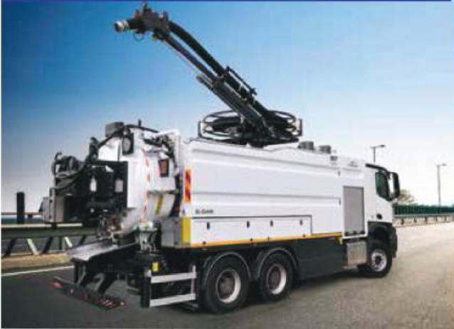
COMBINED SEWER JETTING AND CLEANING
